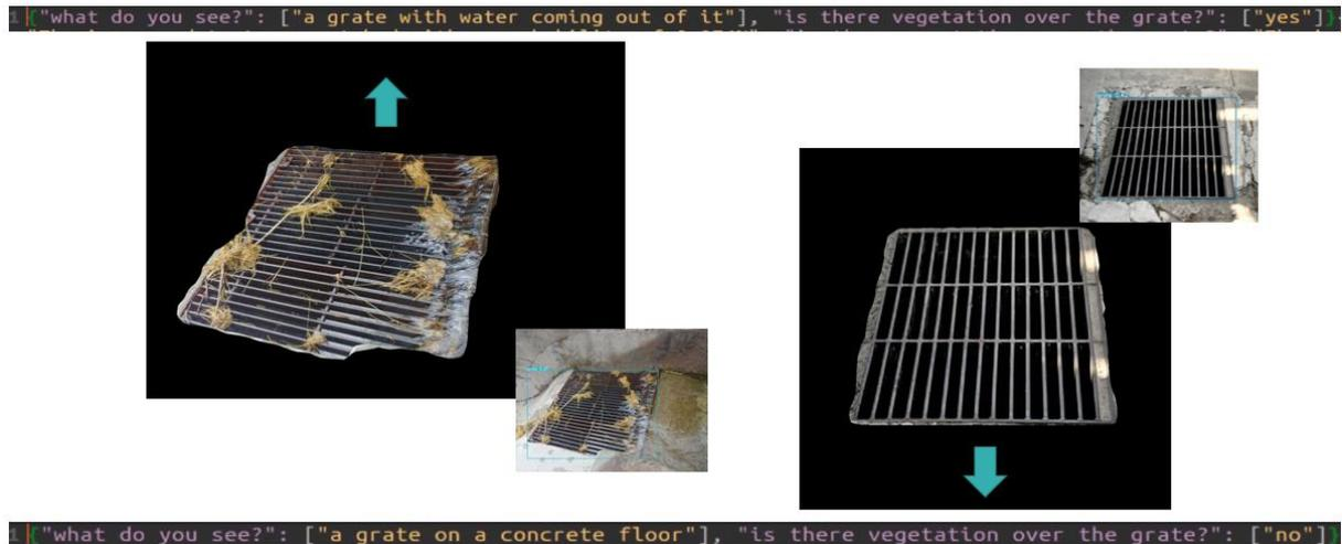
Figure 21: BLIP-2 grate clogging status image interrogation.
