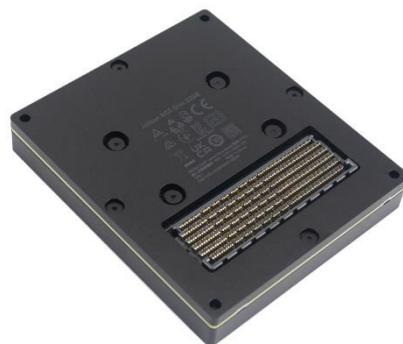
**Figure 31: NVIDIA Jetson AGX Orin 32GB Module [51].**
