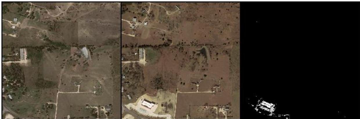
**Figure 7: Example from the LEVIR-CD dataset [16], illustrating detected changes using the CDLR method [22]. The image on the left shows the initial area state, while the middle image shows the later state with newly constructed buildings present in the image. The image on the right displays the predicted changes with CDLR method.**
