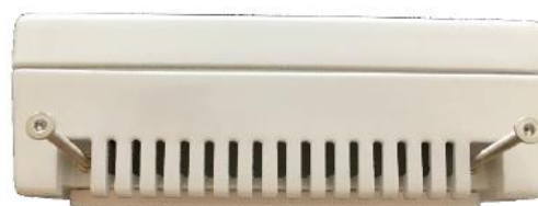
Figure 21: View of the bottom of the terminal with the screws ready for mounting
