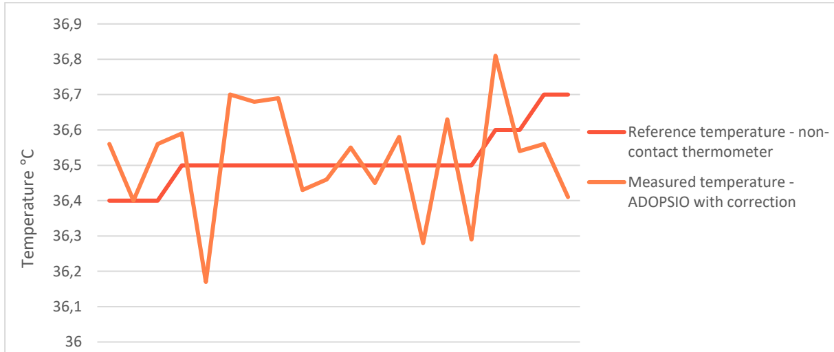
Figure 33: Comparison of body temperature measured with a non-contact thermometer and SUNRISE with correction of the resulting temperature.
