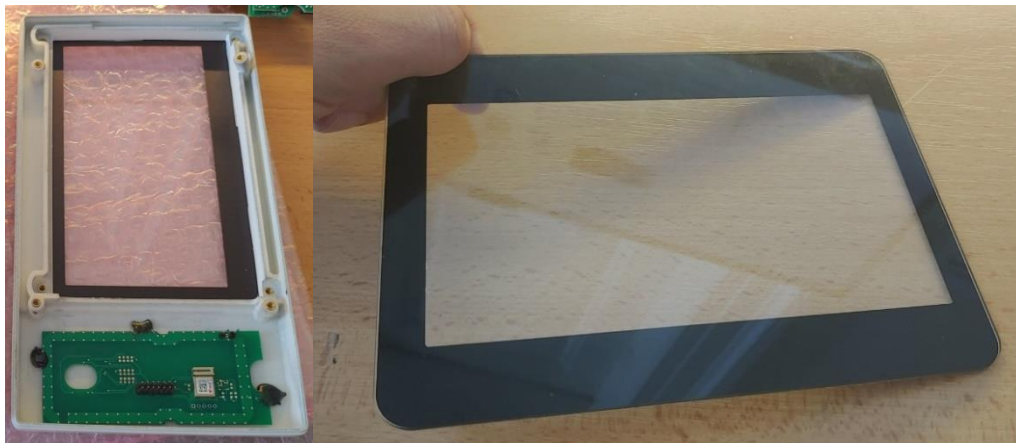
Figure 22: Slot in terminal cover for display, plexiglass with black frame
