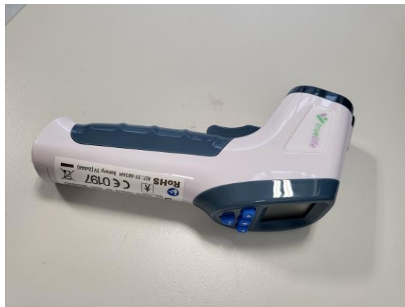
Figure 32: TrueLife Q7 non-contact thermometer for measuring human skin temperature.
