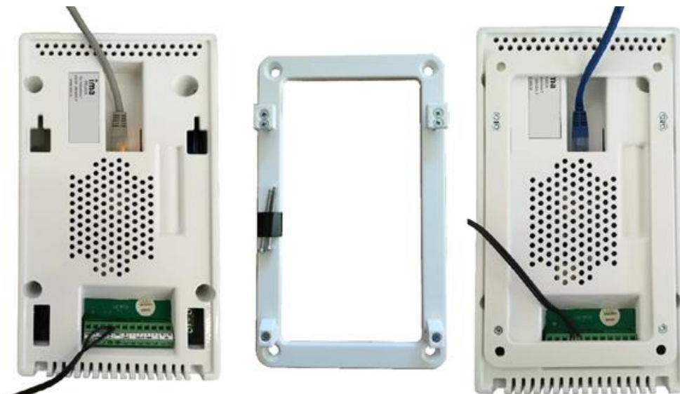
Figure 25: Terminal from the back, mounting frame, mounted frame on the terminal
