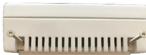
Figure 23: View of the bottom of the terminal with the screws ready for mounting
