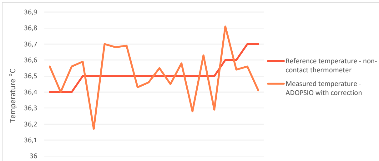
Figure 35: Comparison of body temperature measured with a non-contact thermometer and SUNRISE with correction of the resulting temperature.
