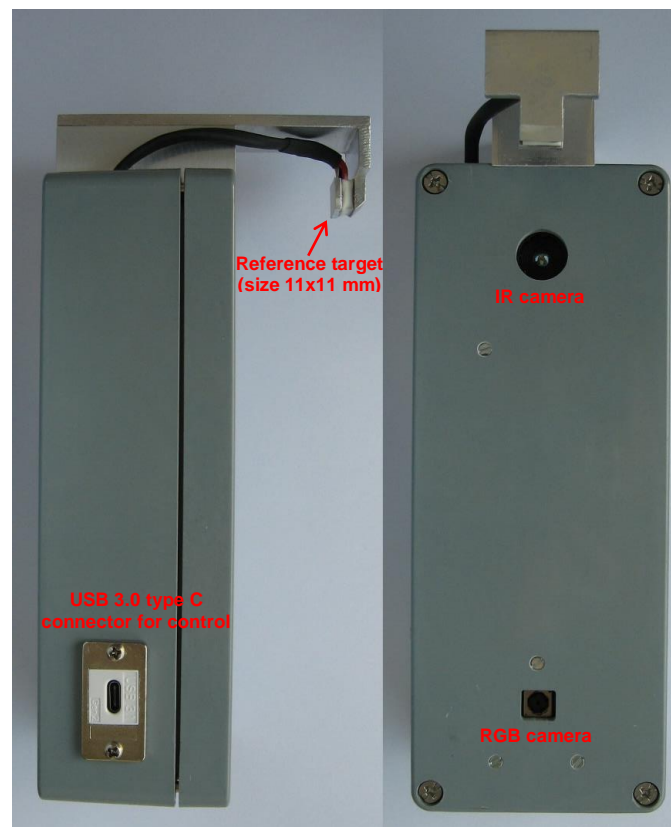
Figure 12: External view of a working sample of the temperature measurement module
