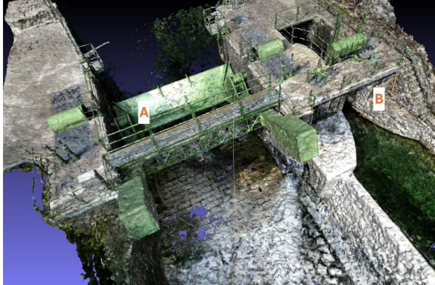
Figure 23: HDE dam 3D mesh measurement estimation. Orange line (A) represents bridge longitude measurement; Orange line (B) represents stair height measurement.
