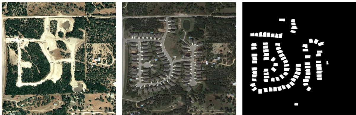
Figure 3: Illustration of LEVIR-CD dataset [8]. Left and middle show images taken at two different times. Right image is labelled with building changes.
